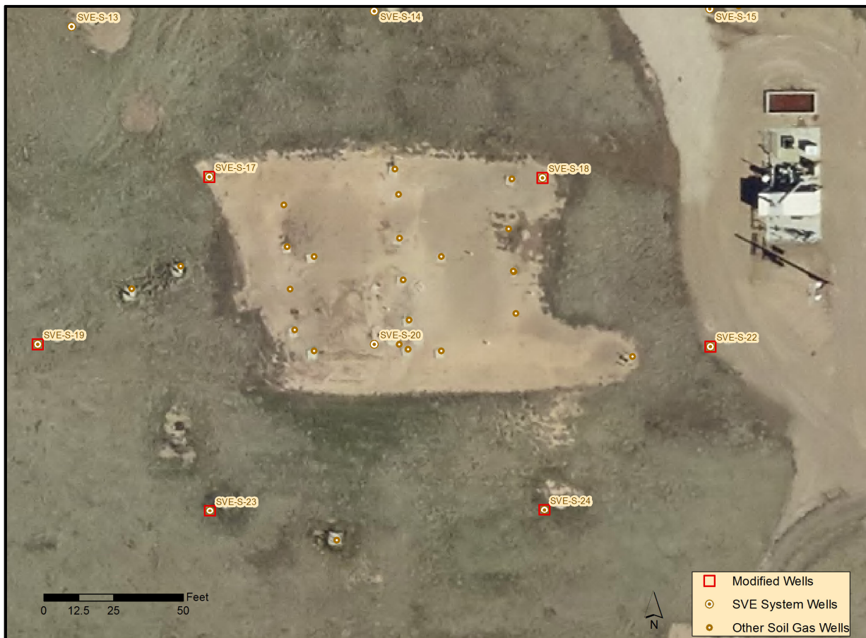
Fig. 1-4. Burning Ground SVE System wells and modifications.
