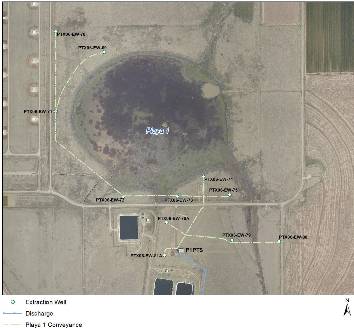
Figure 4.2. P1PTS Extraction Wells and Conveyance Lines
