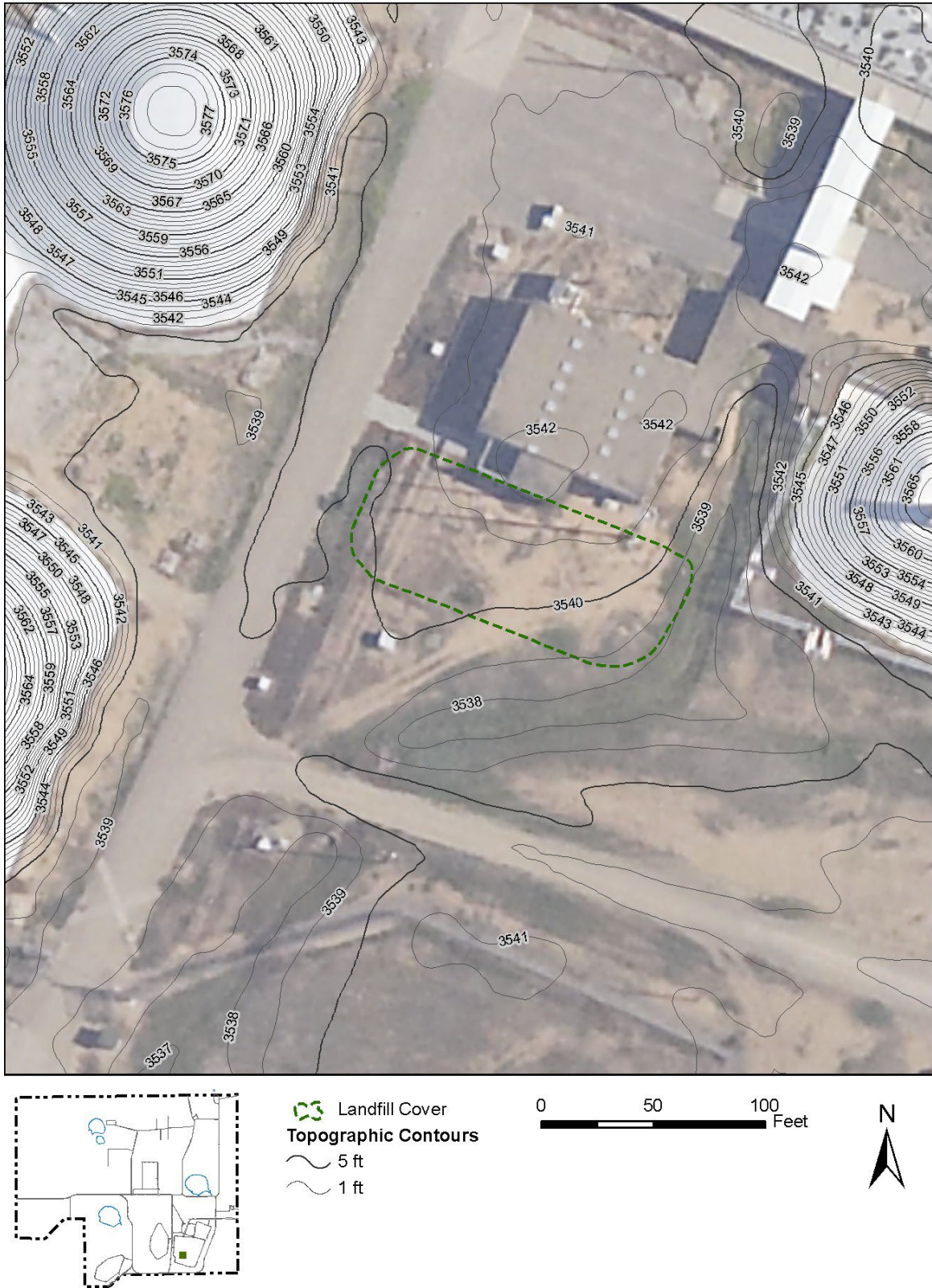
Figure 11. Baseline Survey of Cover for Landfill 6 (SWMU 57)
