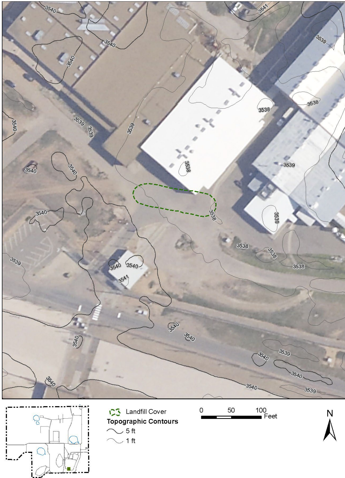
Figure 29. Baseline Survey of Cover for Original Sanitary Landfill (SWMU 68a North)
