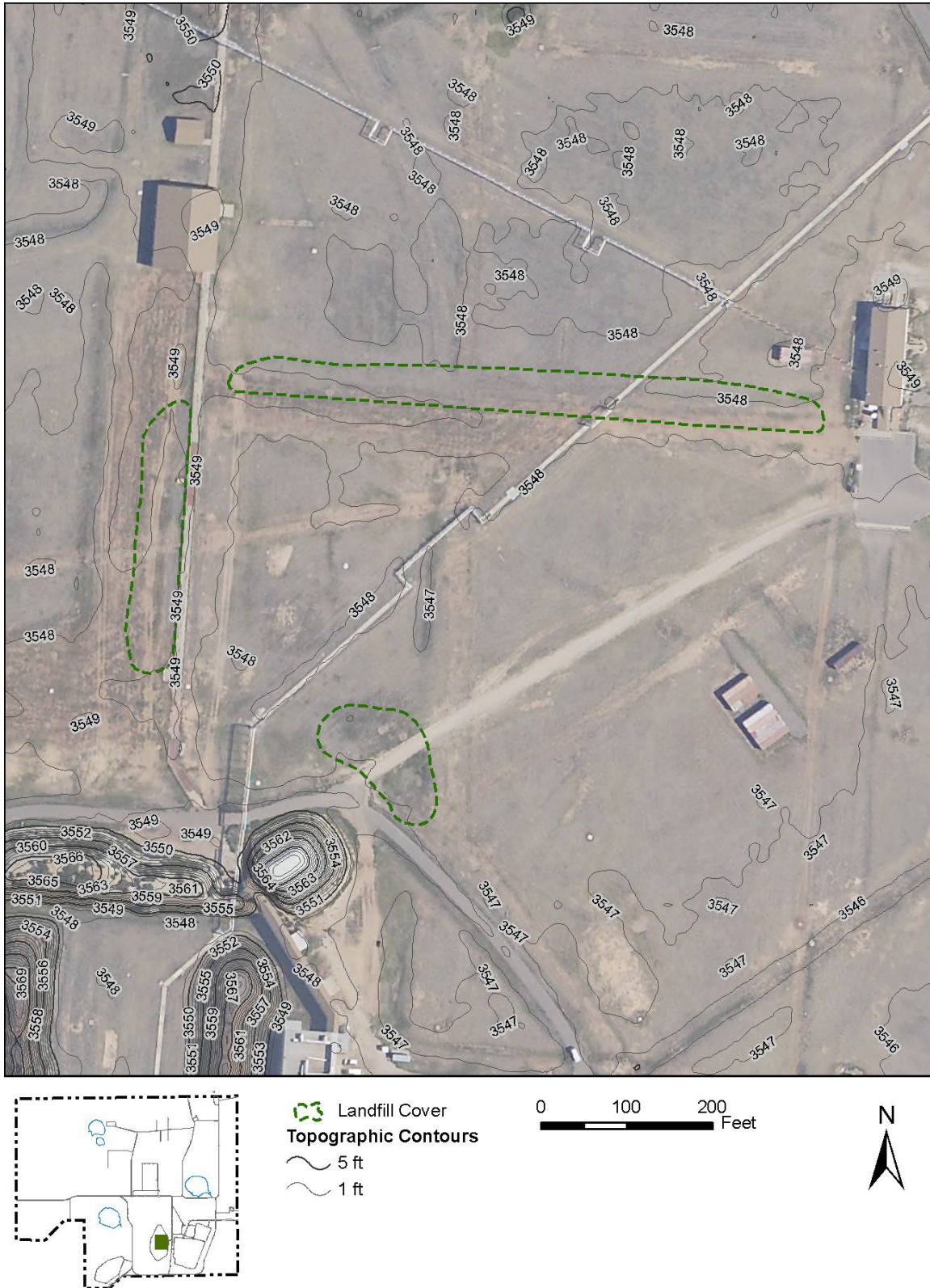
Figure 7. Baseline Survey of Covers for Landfills 9 and 10 (SWMUs 60 & 61)
