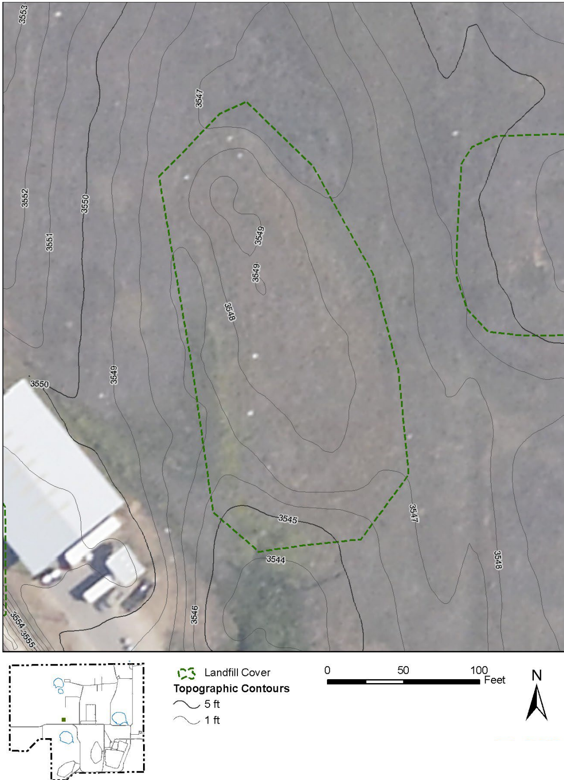
Figure 44. Baseline Survey of Cover for Landfill 12 (SWMU 63)
