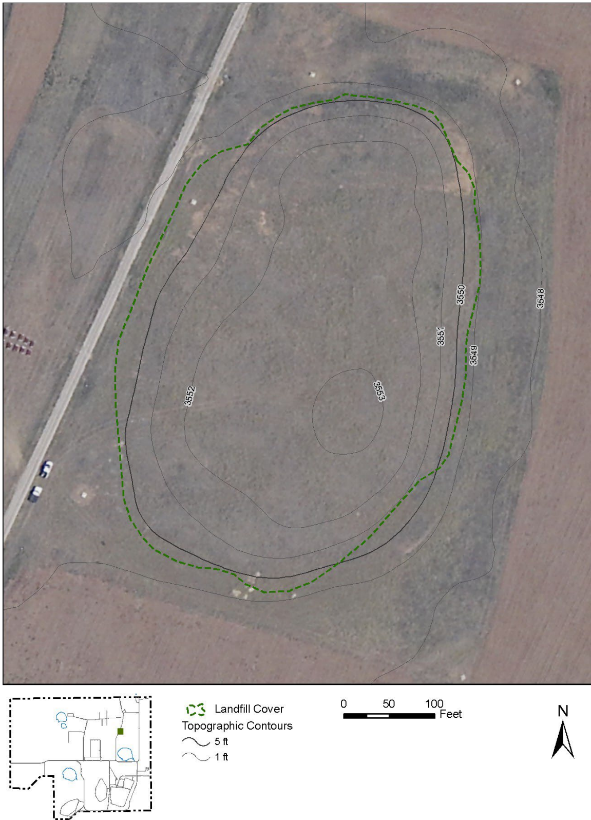
Figure 31. Baseline Survey of Cover for General Purpose Sanitary Landfill 1 (SWMU 68b)
