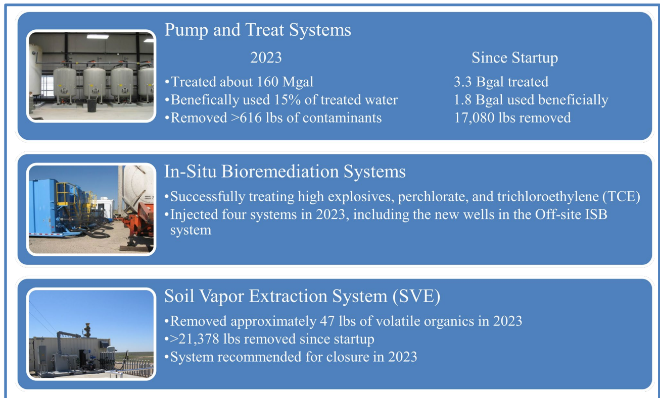
Fig. 3.14. Major Milestones for 2023 remedial actions.
